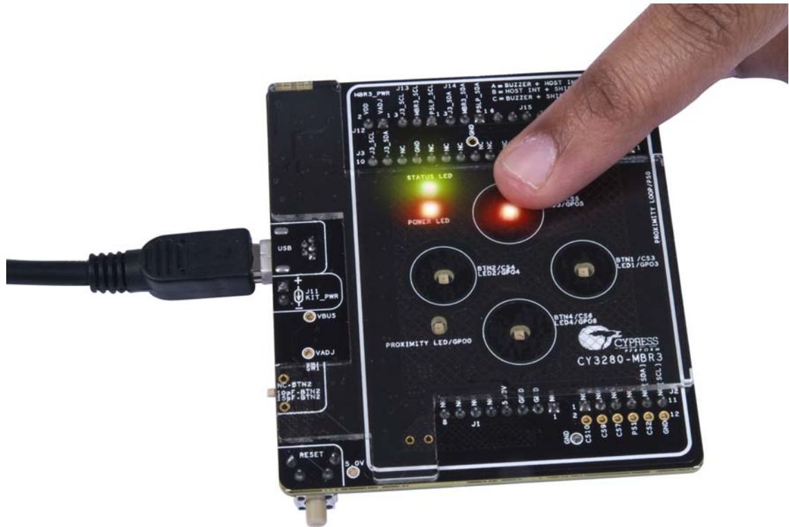
Figure 5-15. Auto-Reset Feature - LED Output on Button Touch
