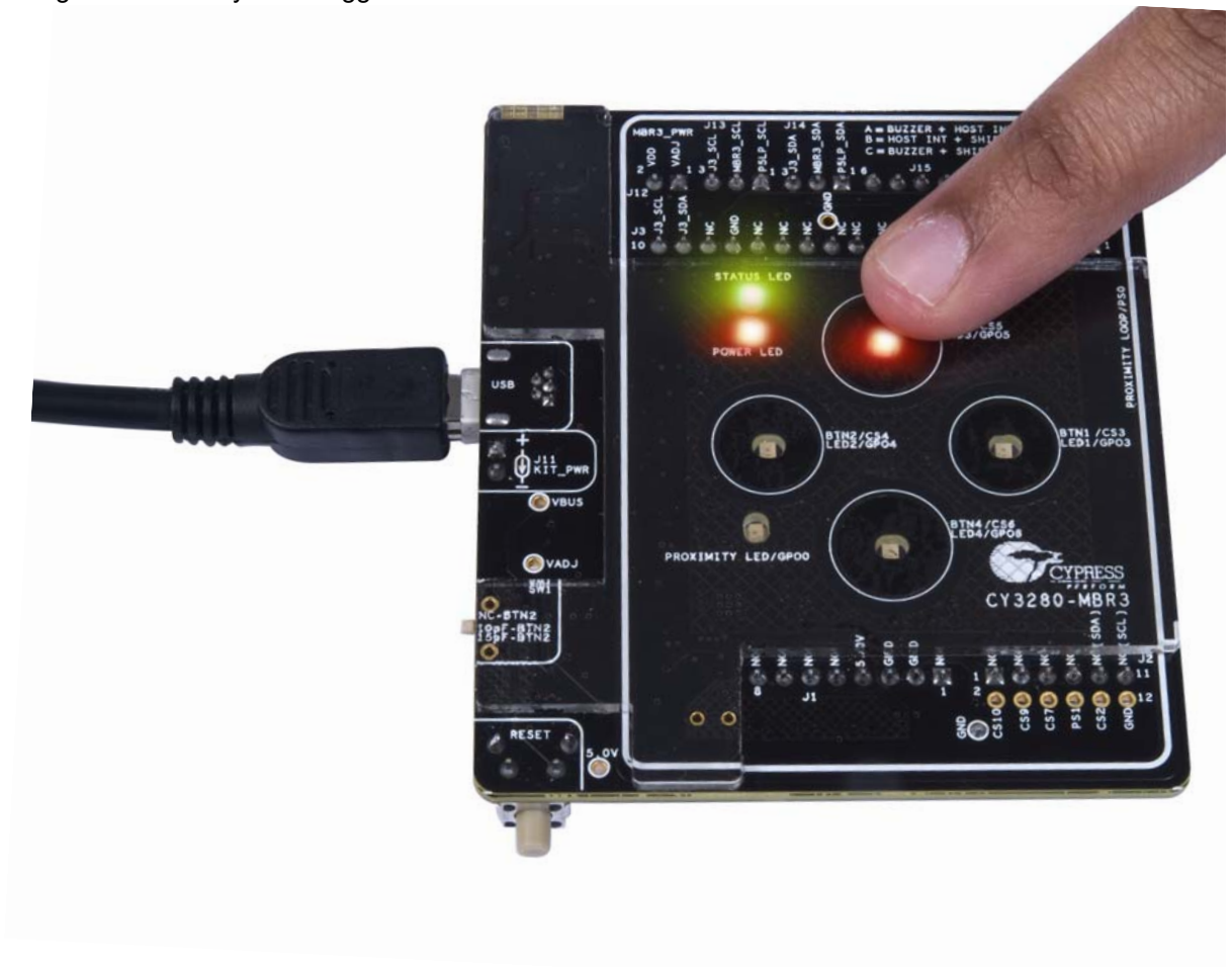
Figure 5-6. Verify LED Toggle Feature
