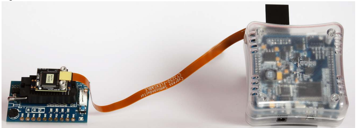
Figure 3-7. Flex Pod Connected to ICE-Cube Pod
