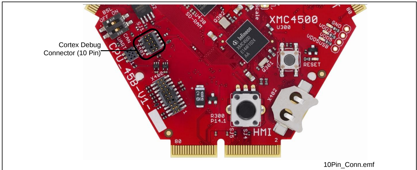
Figure 12 Cortex Debug Connector (10-pin) Layout
