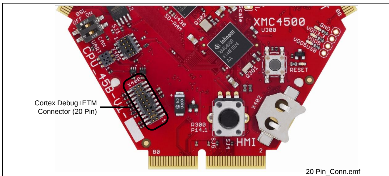
Figure 14 Cortex Debug+ETM Connector (20-pin) Layout
