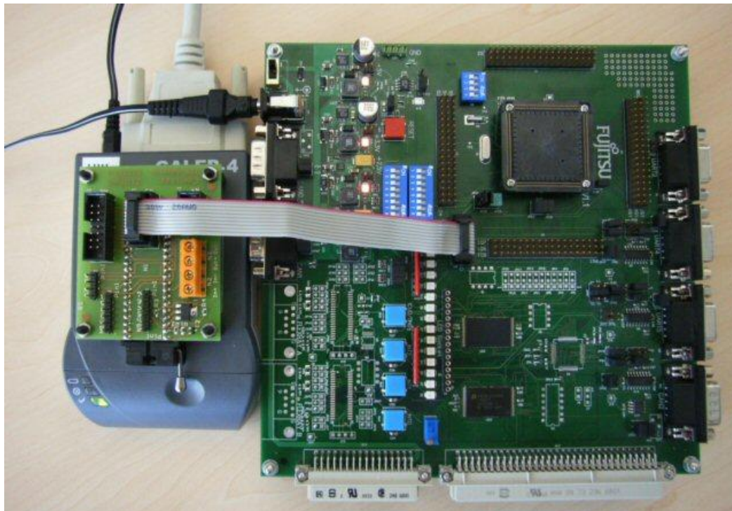
Figure 5-7: Serial Synchronous Programming on SK-91F467D-208PFV
