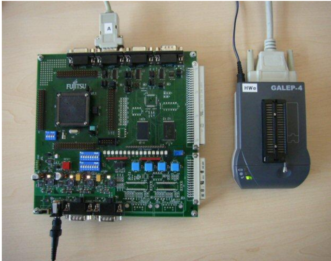
Figure 5-9: Serial Asynchronous Programming with GALEP-4 Programmer
