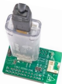
Figure 121. CYBLE-022001-EVAL Using CY8CKIT-002 MiniProg3
