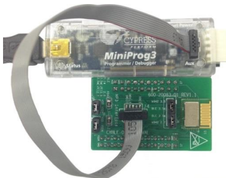
Figure 139. CYBLE-014008-EVAL Using CY8CKIT-002 MiniProg3 and 10-Pin Ribbon Cable
