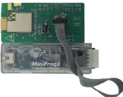
Figure 148. CYBLE-212006-EVAL Using CY8CKIT-002 MiniProg3 and 10-Pin Ribbon Cable
