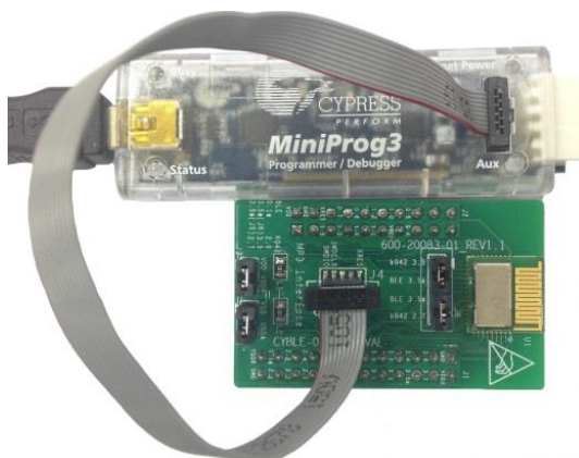
Figure 154. CYBLE-224116-EVAL Using CY8CKIT-002 MiniProg3 and 10-Pin Ribbon Cable
