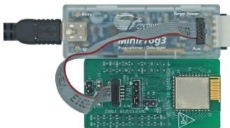
Figure 136. CYBLE-212020-EVAL Using CY8CKIT-002 MiniProg3 and 10-Pin Ribbon Cable
