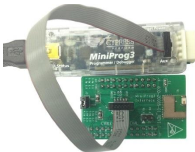
Figure 127. CYBLE-222014-EVAL Using CY8CKIT-002 MiniProg3
