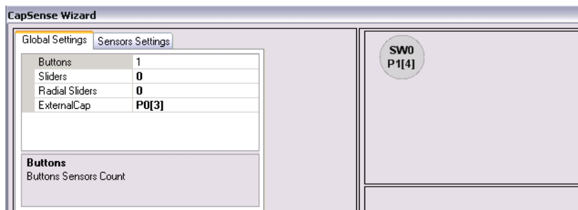
Figure 4-5. CapSense Wizard (Sensor Pin = P1[4], C INT Pin = P0[3])
