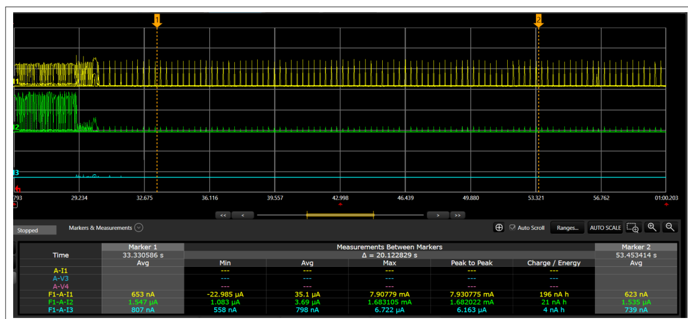
Figure 20 Deep Sleep connection idle with 300 ms connection interval
