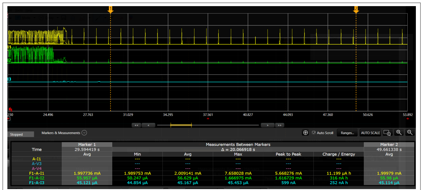
Figure 18 Sleep connection idle with 1 s connection interval
