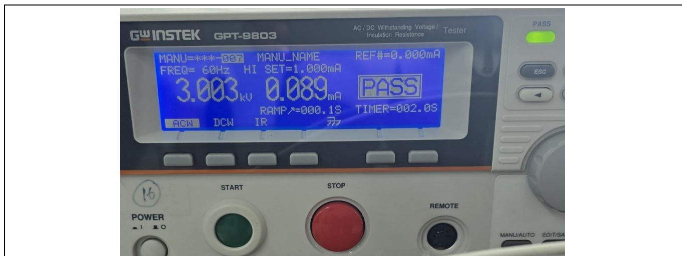
Figure 71 Hi-POT test result
