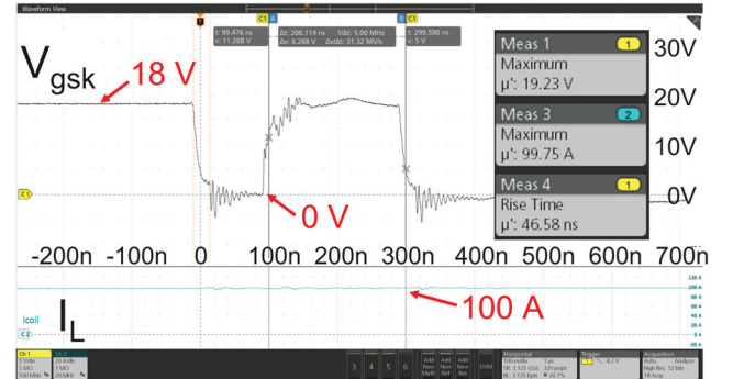
Fig. 12. A detailed image of the gate-to-kelvin-source (black waveform; C1) showing good controllability of the MOSFETs with uni-polar gate driving without pronounced gate ringing. The turquoise curve ( I_L ) shows the current trough the inductor reaching \sim 100 A after 40 \mu s (an aircoil with 200 \mu H was used as load).
