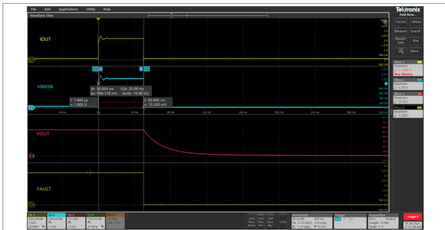
Figure 13 Overcurrent fault being triggered after 50 ms of V_{IMON} reaching ~1.0025 V; R_{IMON} = 27.5 \text{ k}\Omega
