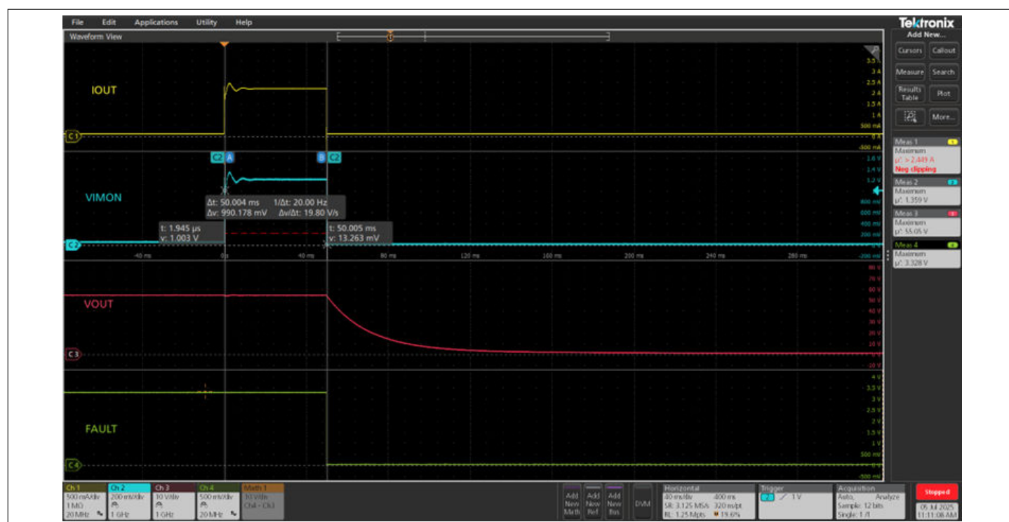
Figure 12 Overcurrent fault being triggered after 50 ms of V_{IMON} reaching \sim 1.0025 V; R_{IMON} = 27.5 k \Omega
