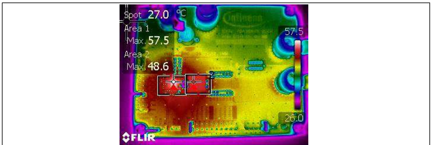
Figure 22 Thermal image at 20 A load TDA38820 = 58°C, L = 49°C, f sw = 600 kHz, T a = 25°C, natural convection
