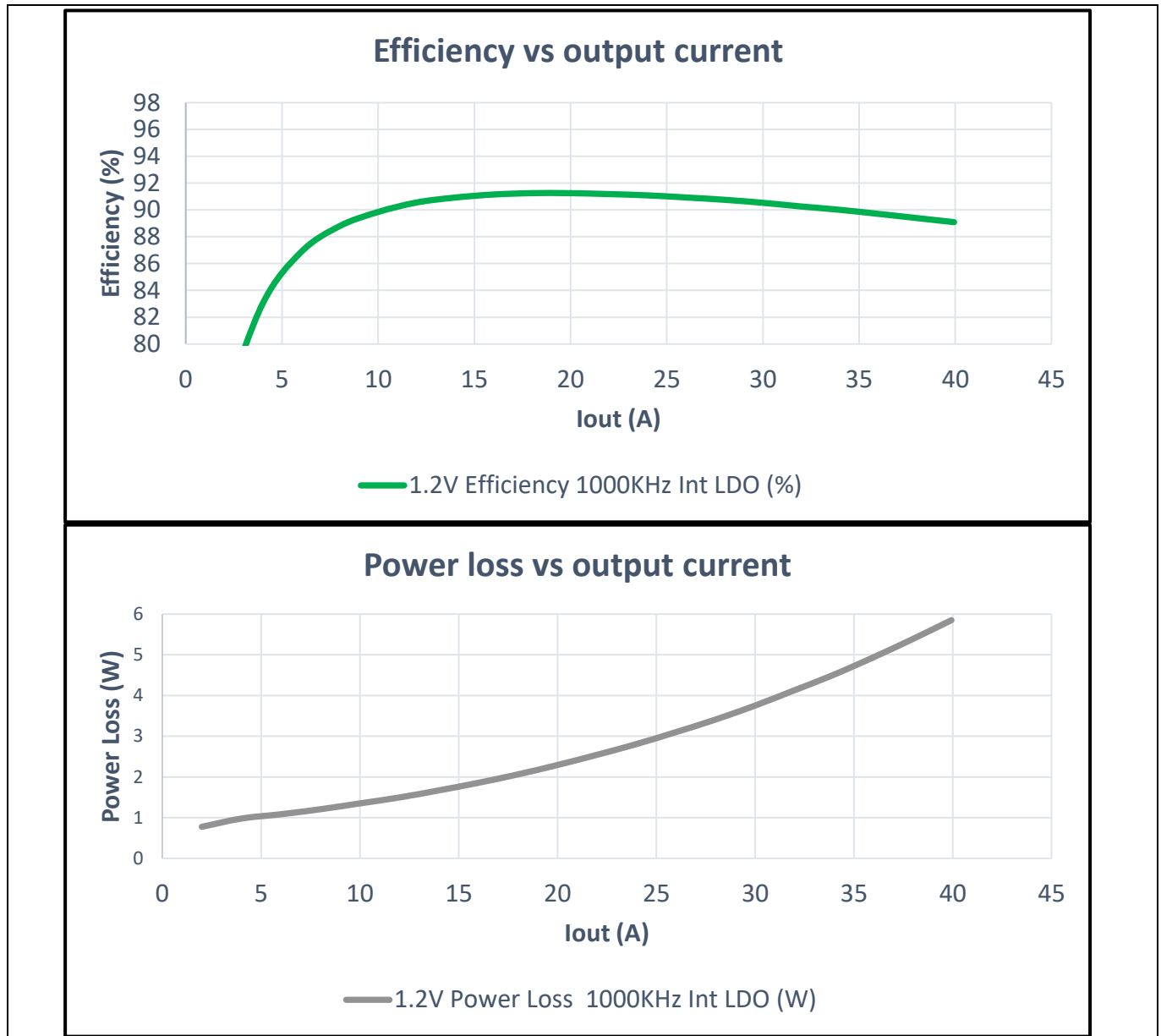
Figure 9 Typical efficiency and power loss curves, PV_{in} = V_{in} = 12\text{ V} , V_{out} = 1.2\text{ V} , F_{sw} = 1000\text{ kHz}
