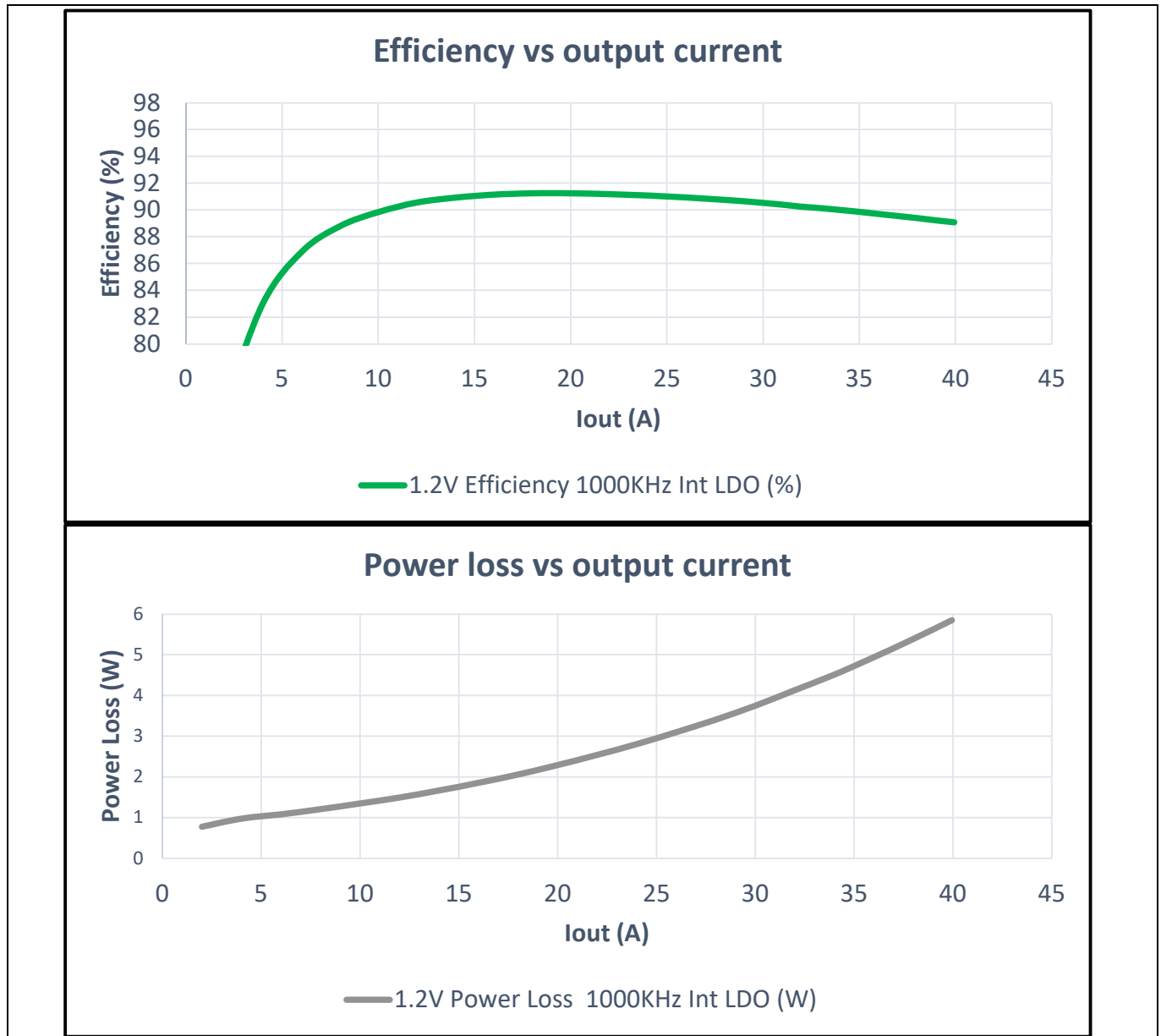
Figure 9 Typical efficiency and power loss curves, PV_{in} = V_{in} = 12 V, V_{out} = 1.2 V, F_{sw} = 1000 kHz
