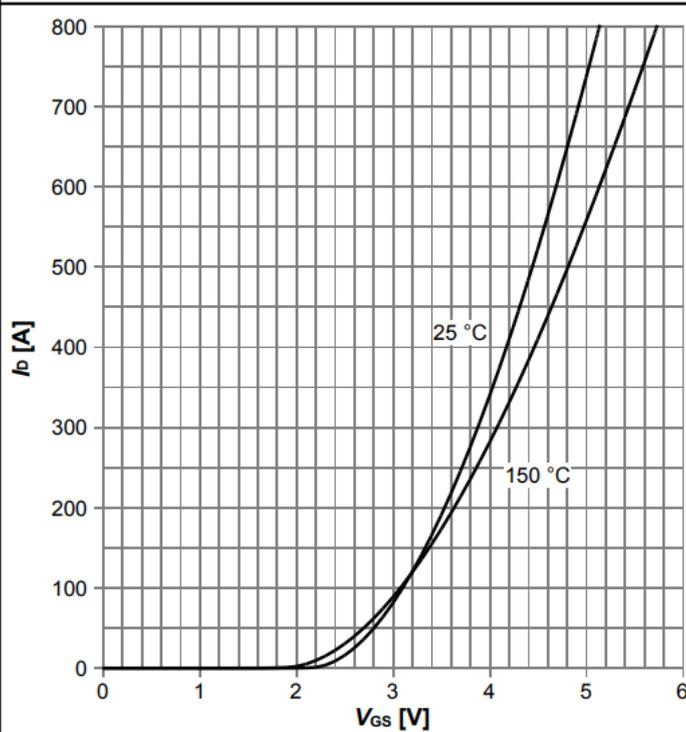
$I_D = f(V_{GS}), |V_{DS}| > 2|I_D|R_{DS(on)max};$  parameter:  $T_j$
