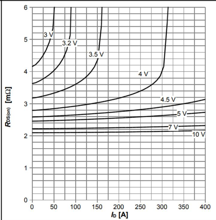
$R_{DS(on)} = f(I_D), T_j = 25\text{ °C};$  parameter:  $V_{GS}$
