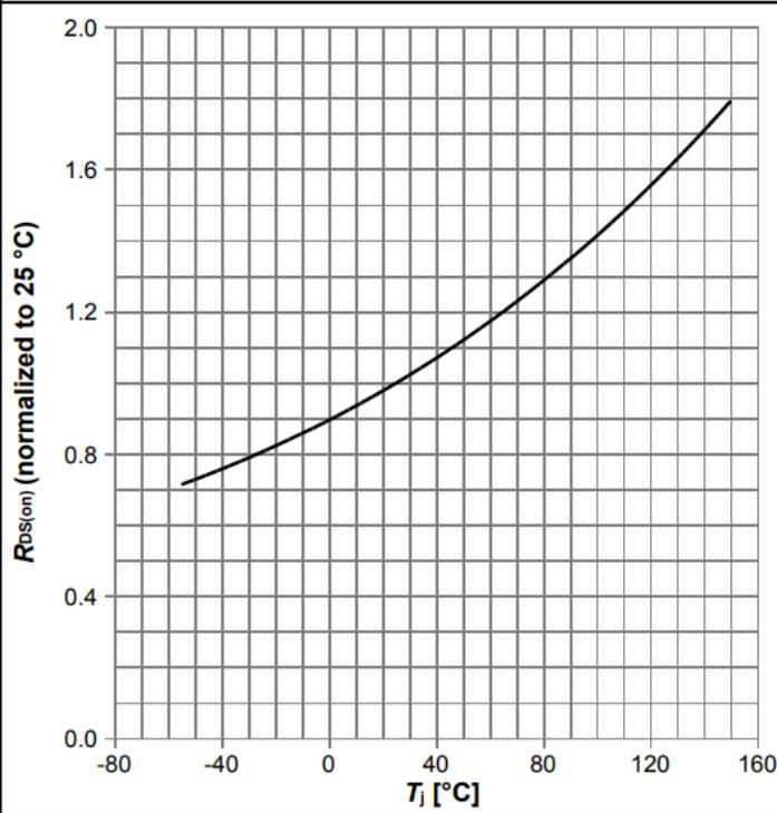
$R_{DS(on)}=f(T_j)$ ,  $I_D=50$  A,  $V_{GS}=10$  V
