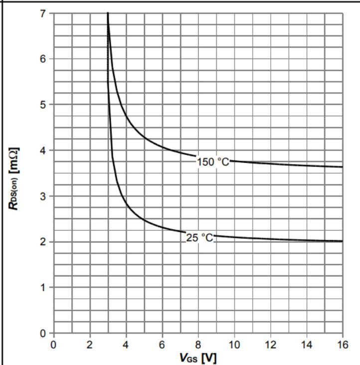
$R_{DS(on)} = f(V_{GS}), I_D = 50\text{ A};$  parameter:  $T_j$
