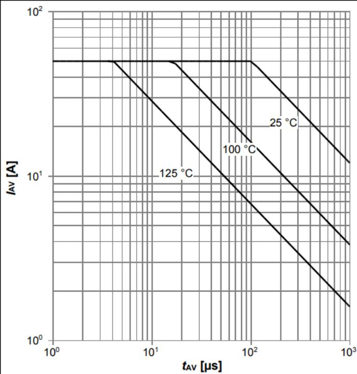
$I_{AS}=f(t_{AV}); R_{GS}=25 \Omega$ ; parameter:  $T_{j,start}$
