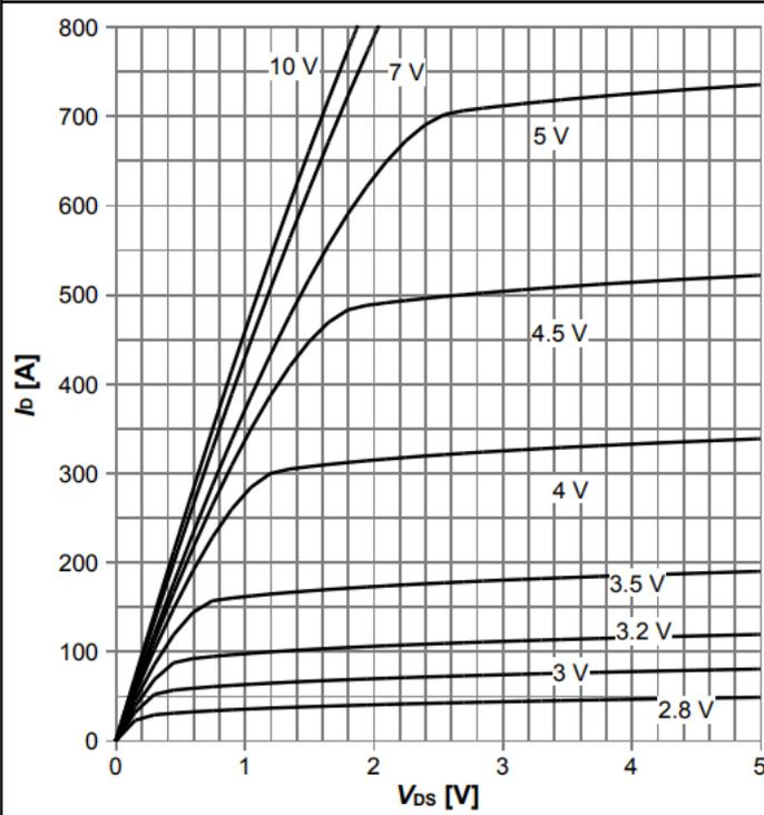
$I_D = f(V_{DS}), T_j = 25\text{ °C};$  parameter:  $V_{GS}$
