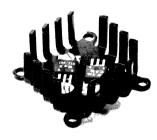
(c) Type 689-75 B-4 heatsink gives 1A continuous rating for IRF710 with natural convection cooling in 40°C ambient.
