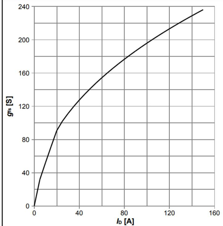
$g_{fs} = f(I_D); T_J = 25\text{ }^\circ\text{C}$
