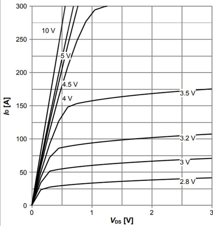
$I_D = f(V_{DS}); T_J = 25\text{ }^\circ\text{C};$  parameter:  $V_{GS}$
