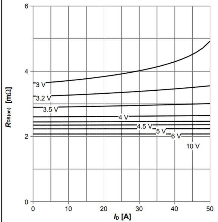
$R_{DS(on)} = f(I_D); T_J = 25\text{ }^\circ\text{C};$  parameter:  $V_{GS}$
