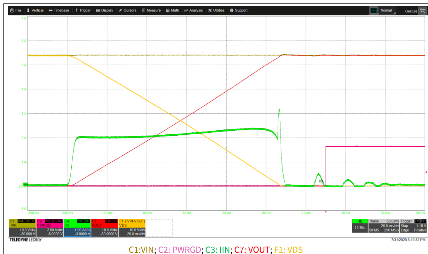
Figure 47 Reference board startup waveform
