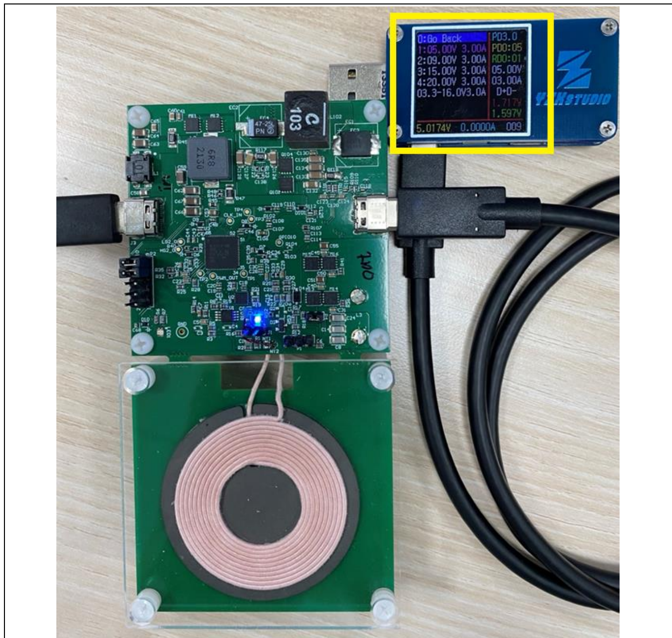
Figure 27 WLC1115 Qi PTx as standby, CCG7SC USB-C PD output have all of capability 60 W
