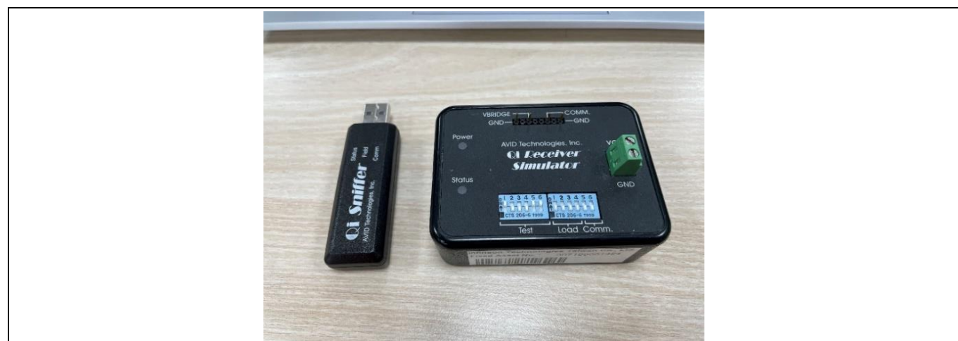
Figure 4 Confirm Qi PTx capabilities using Qi Sniffer and Qi Receiver Simulator
