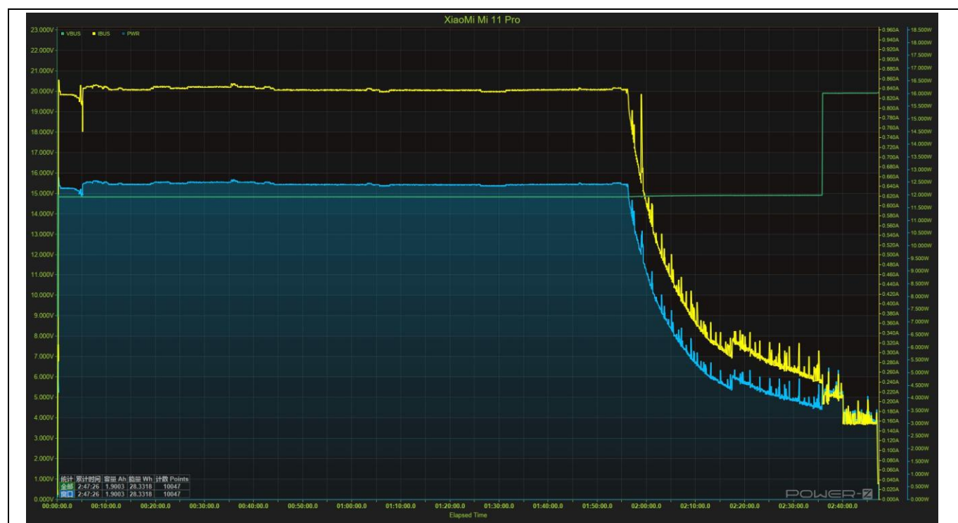
Figure 13 Charge cycle results for the Xiaomi Mi 11 pro (Green: VBUS, Yellow: IBUS, Blue: Watt)
