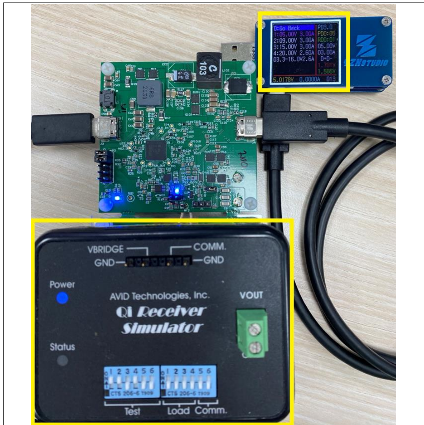
Figure 28 Reserve 8 W for WLC1115 Qi PTx BPP, share remaining 52 W to CCG7SC USB-C PD
