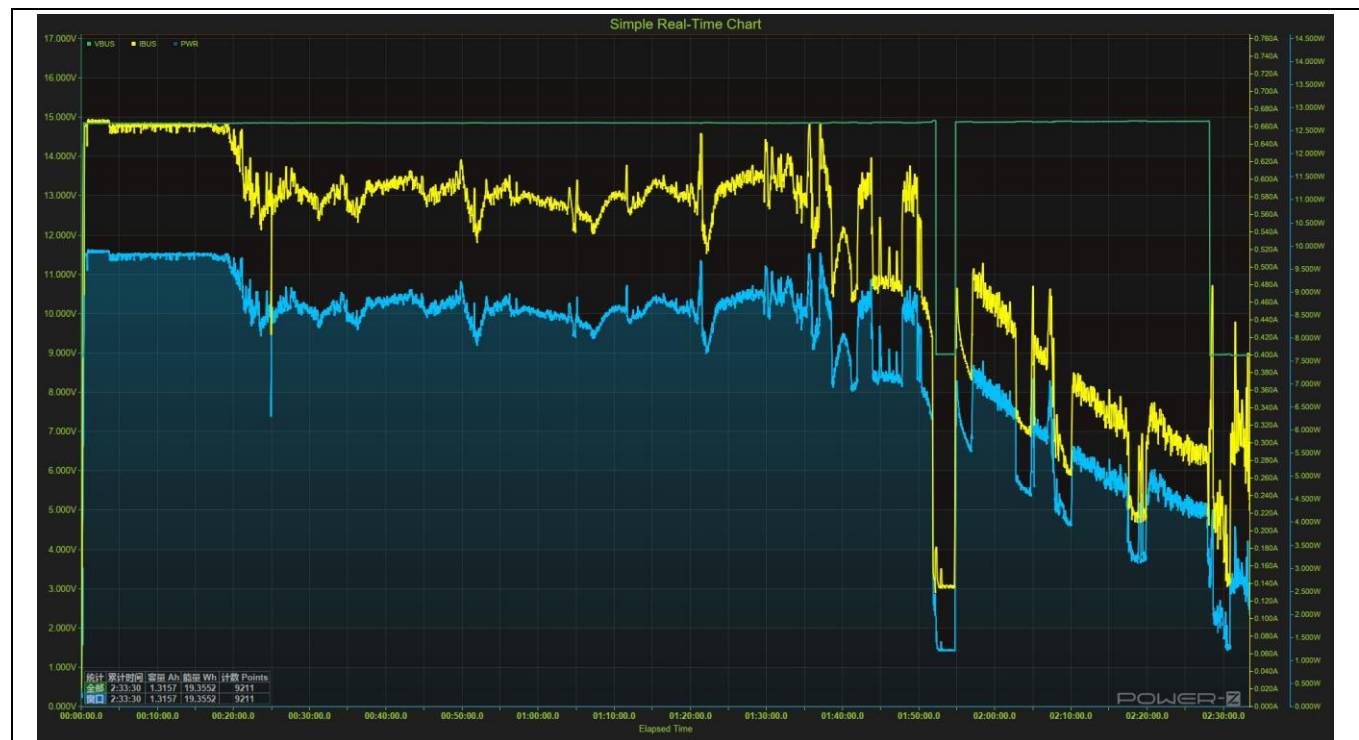
Figure 16 Charge cycle results for Apple iPhone 13 (Green: VBUS, Yellow: IBUS, Blue: Watt)
