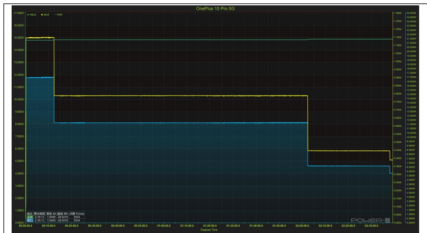
Figure 15 Charge cycle result for OnePlus 10 Pro 5G (Green: VBUS, Yellow: IBUS, Blue: Watt)
