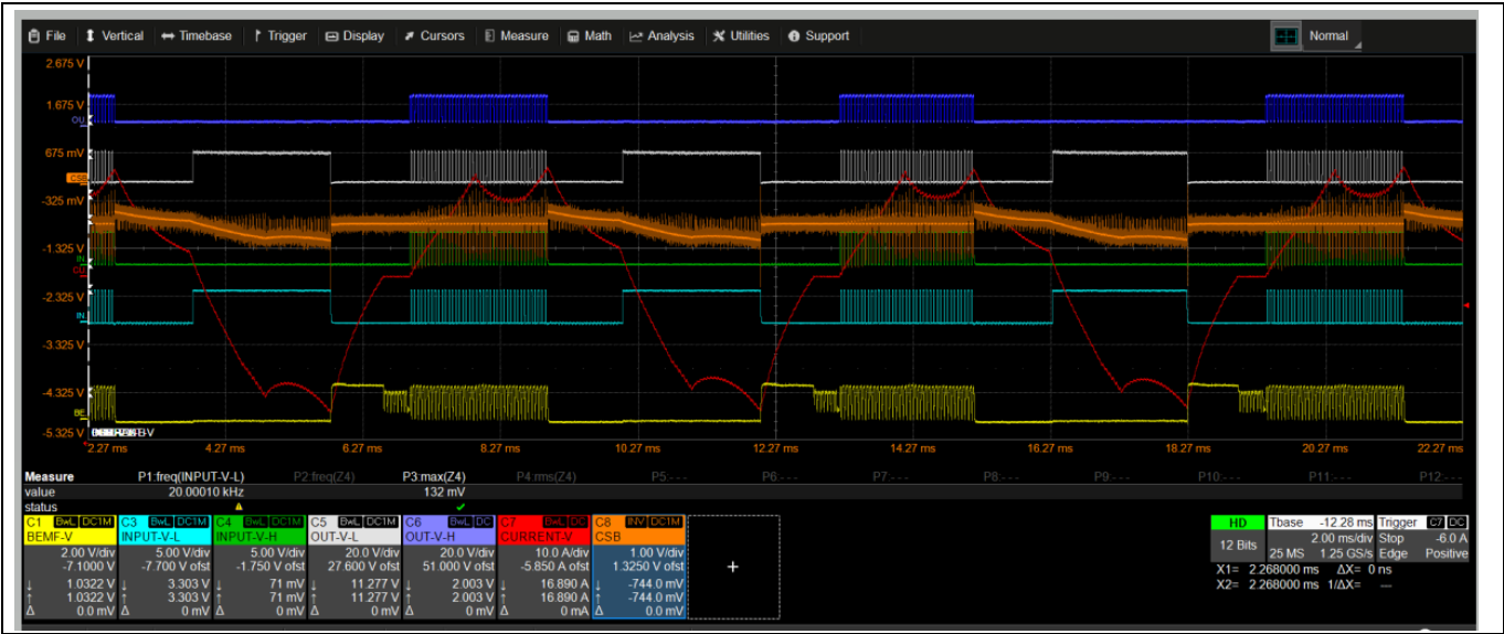
Figure 41 BEMF_V (yellow), INPUT_V_L (cyan), INPUT_V_H (green), V_{GS\_LS} (gray), V_{GS\_HS} (blue), I_{PHASE\_CURRNTN} (red), I_{PHASE\_B} (orange) (signals after the internal amplifier)
