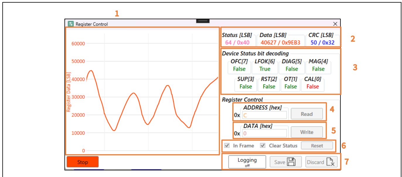
Figure 42 SPI Readout view – Register Control
