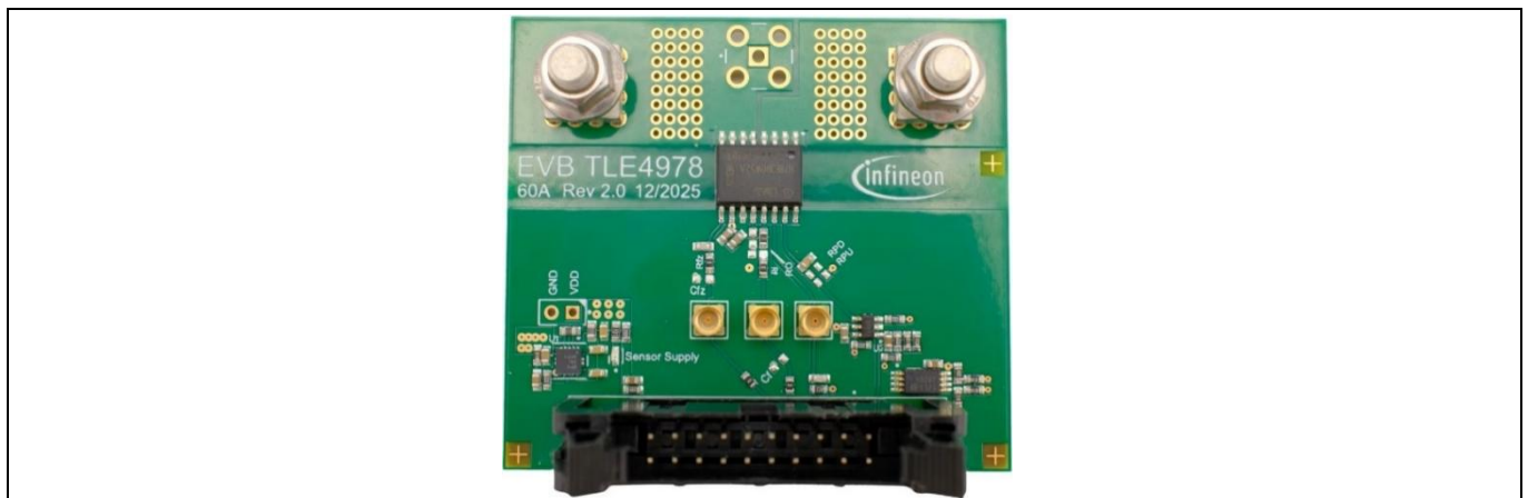
Figure 1 XENSIV™ TLE4978 Current Sensor Evaluation Board
