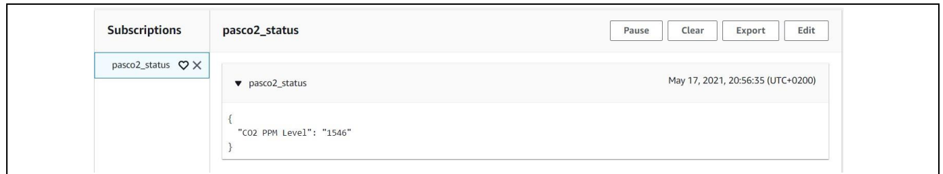
Figure 12 CO 2 PMM level value on the MQTT broker
