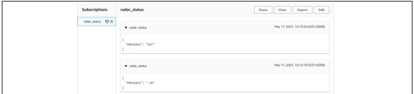
Figure 12 Event detection message from MQTT
