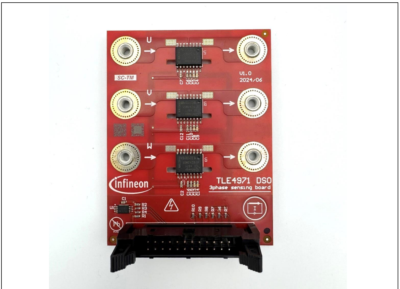
Figure 1 TLE4971 EVAL 50A, three phase measurement board
