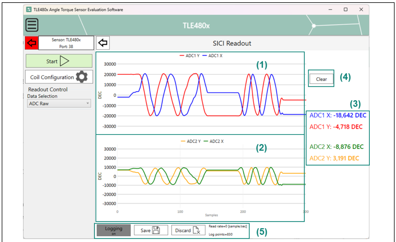
Figure 20 SICI Readout view, ADC Raw
