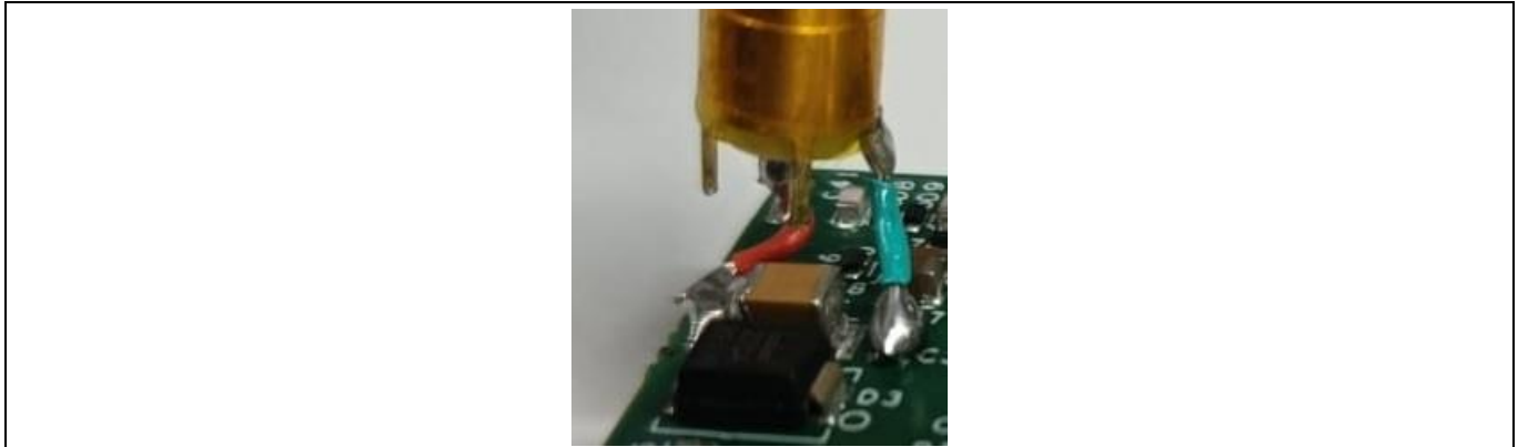
Figure 19 Output voltage ripple measurement test setup
