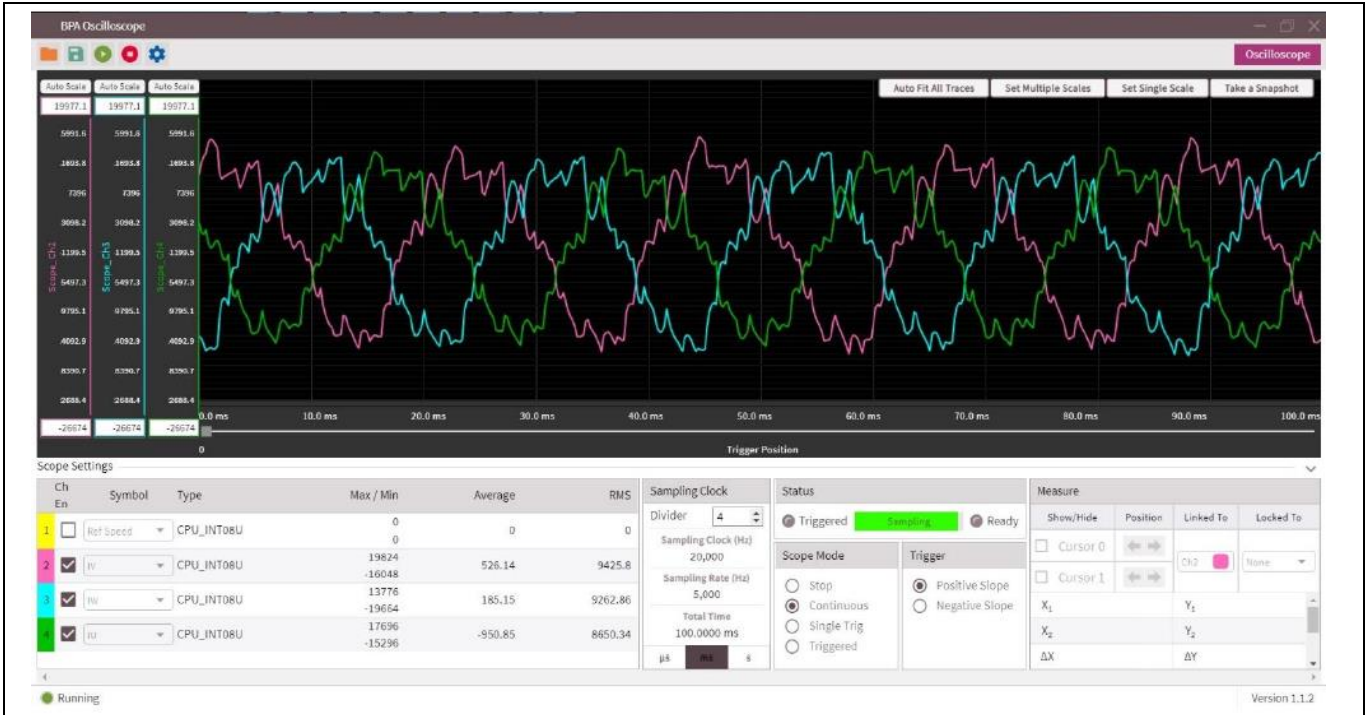
Figure 28 Oscilloscope view showing the phase currents; I_u (green), I_v (red), I_w (blue)
