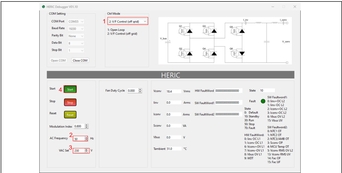
Figure 43 Using the converter in V/F control mode
