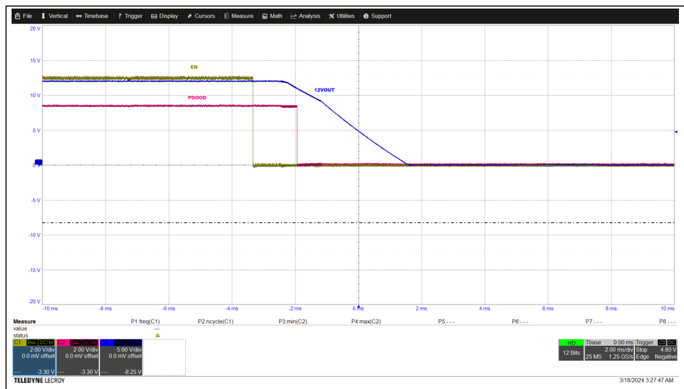
Figure 32 Shutdown waveform. CH1: EN, CH2: P GOOD , CH3: 12 V output
