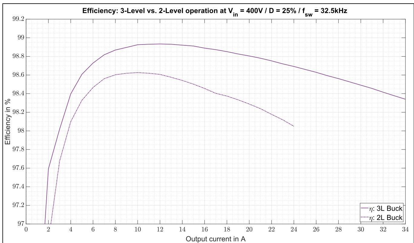
Figure 40 Comparison of efficiency curves between 2-level and 3-level operation
