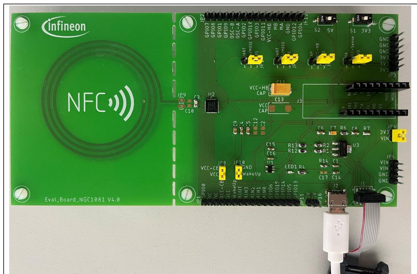
Figure 17 rConnection of USB and debugger to the NGC1081
