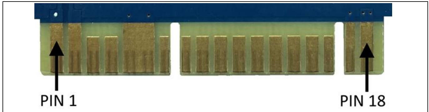
Figure 5 Edge card header with 36 pins (18 pins symmetrical, top and bottom); designed to work with EBC18DCWN-S371 board-to-board receptacle connector
