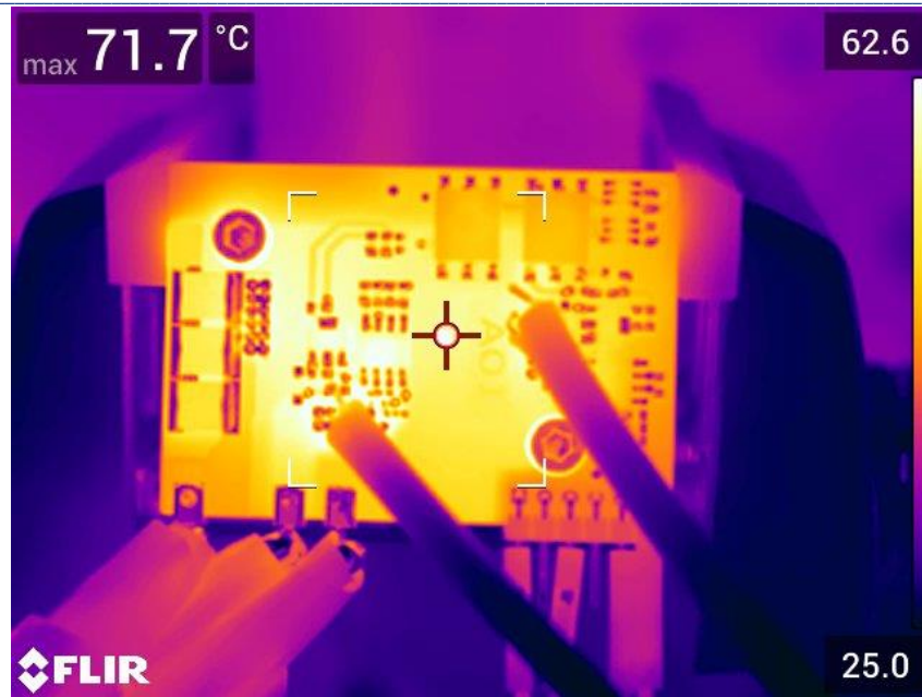
Figure 11 Boost configuration test thermal measurement result
