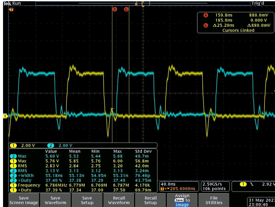
Figure 15 • Oscilloscope Plot Showing Both GS66508B Gate Node Signals at TP8, TP81
