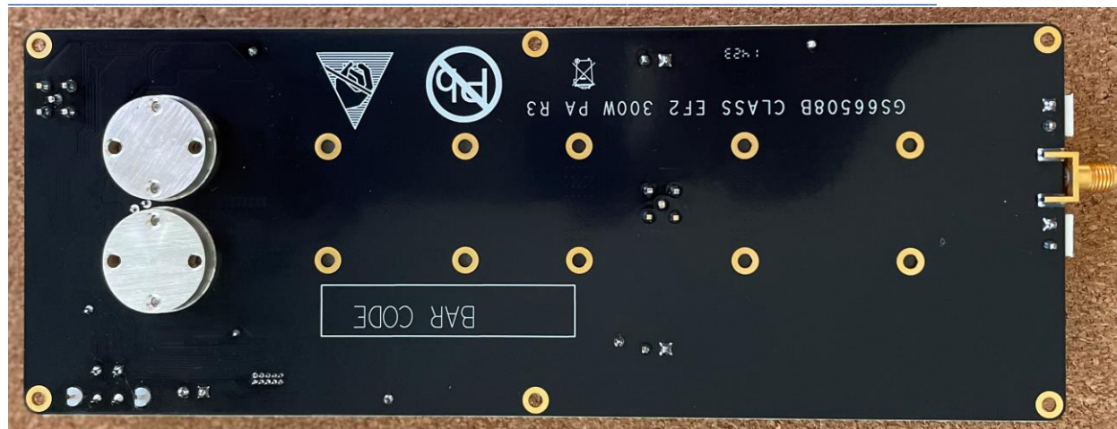
Figure 3 • Bottom side of GSWP300W-EVBPA Evaluation Board Assembly, showing copper coins
