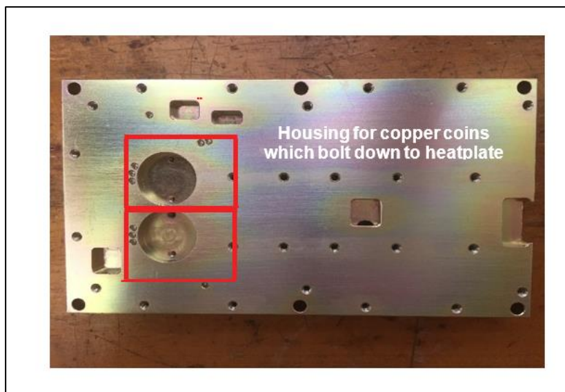
Figure 12 • Aluminum heatplate with housing for two copper coins.
