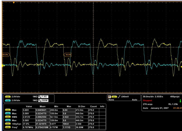
Figure 16 • Oscilloscope Plot Showing Both GS61008P Gate Node Signals at TP8, TP81
