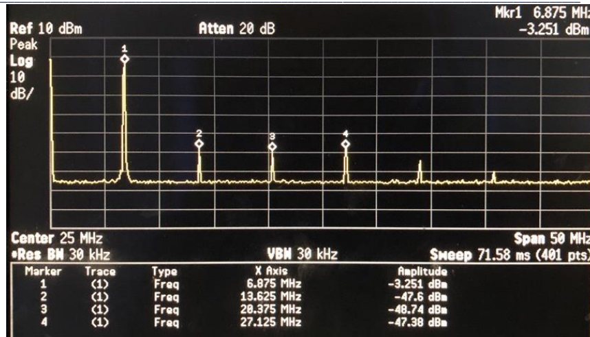
Figure 21 • Spectrum plot of output terminal JP57 SMA after 53.6dB attenuation at 100W output power
