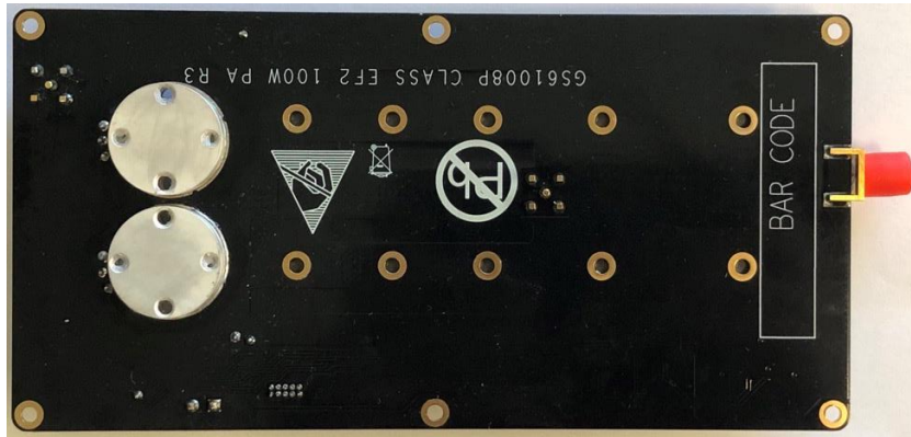
Figure 3 • Bottom side of GSWP100W-EVBPA Evaluation Board Assembly, showing copper coins
