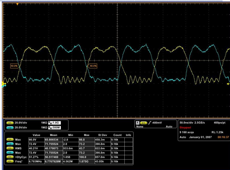
Figure 17 • Oscilloscope Plot Showing Both GS61008P Drain Node Signals
