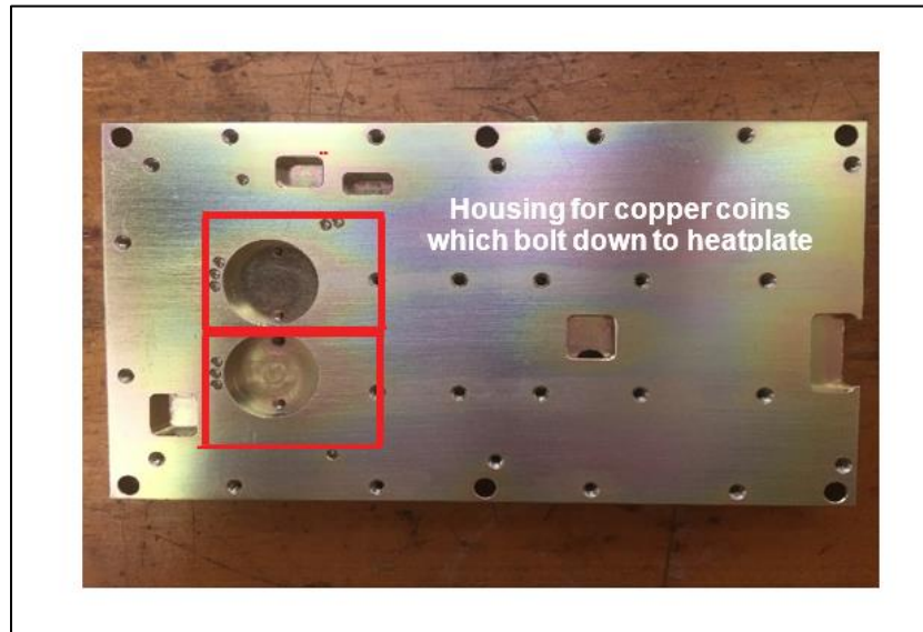
Figure 13 • Aluminum heatsink with housing for two copper coins.
