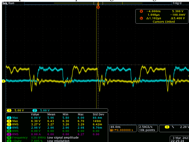
Figure 16 • Oscilloscope Plot Showing Both GS61004B Gate Node Signals at TP8, TP81
