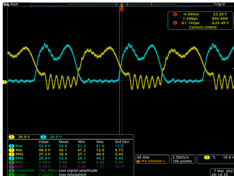
Figure 17 • Oscilloscope Plot Showing Both GS61004B Drain Node Signals
