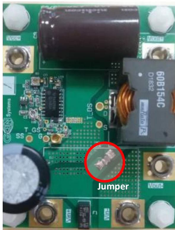
Figure 7 • Current Sensing Jumper Location
