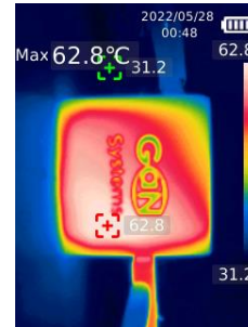
Figure 15. Surface temperature images after 1-hour continuous run at full load with 28V/5A (140W) output
