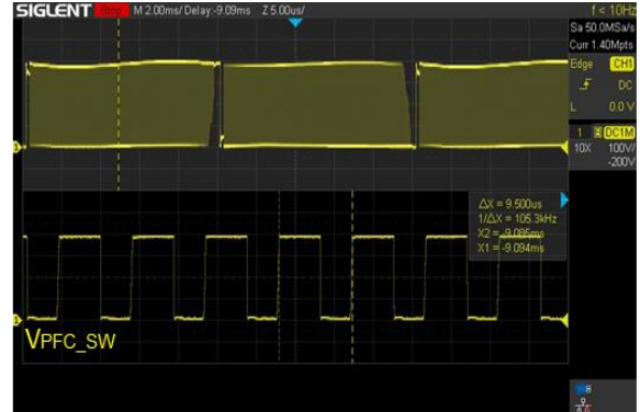
115Vac@28V5A,full Load, sinusoid top freq=105kHz
