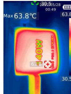
Figure 15. Surface temperature images after 1-hour continuous run at full load with 28V/5A (140W) output
