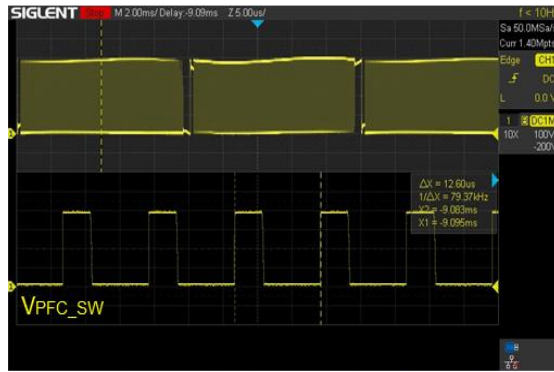
90Vac@28V5A,full Load, sinusoid top freq=75kHz
