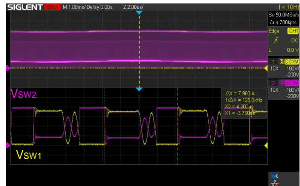
75% Load 28V 3.75A, Freq=125kHz
