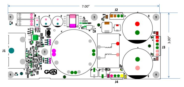
Connector: J3 (Mating JST Connector: VHR-6N; Pin: SVH-41T-P1.1)
