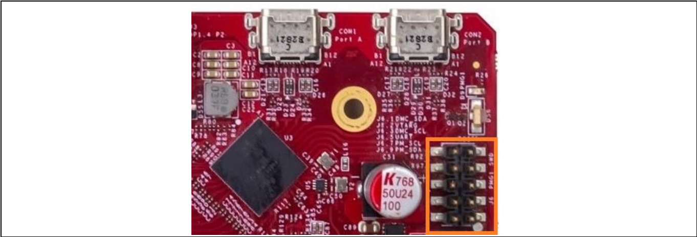
Figure 12 SWD header to program PMG1-S3 using Minipro4 Programmer/Debugger
