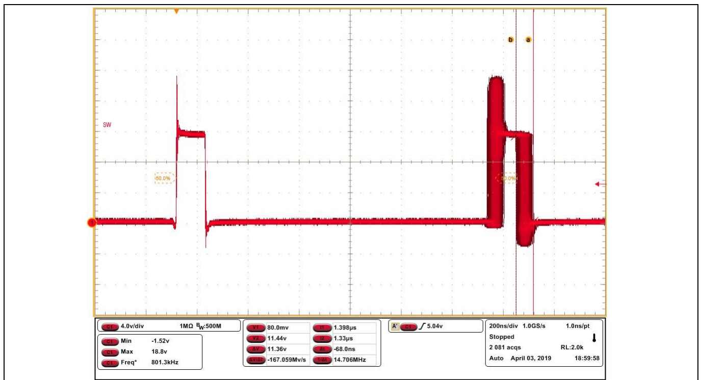
Figure 16 SW node, 30 A load, fsw = 800 kHz
