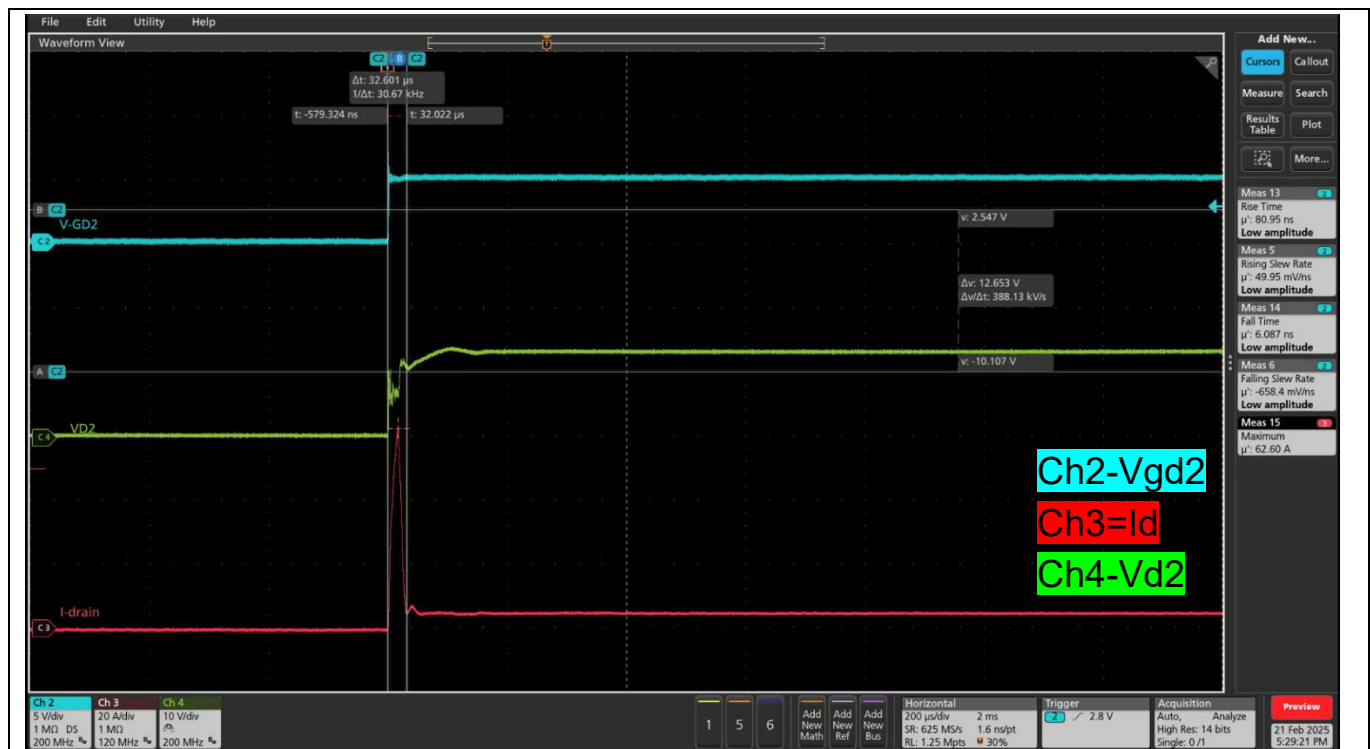
Figure 14 Turn on without RC delay on gate drive path- V_{D1}=20\text{ V} , I_d=5\text{ A} (load), V_{GD2} = 0\text{ V} to 5\text{ V} , I_{d\_max} = 62.6\text{ A} , t_{I_{max}} = 32.6\text{ us}
