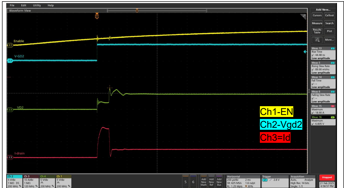
Figure 13 Turn on without RC delay on gate drive path- V_{D1}=5\text{ V} , I_d=10\text{ A} (load), V_{GD2} = 0\text{ V} to 5\text{ V} , I_{d\_max} = 18.9\text{ A} , t_{I_{max}} = 120\text{ us}
