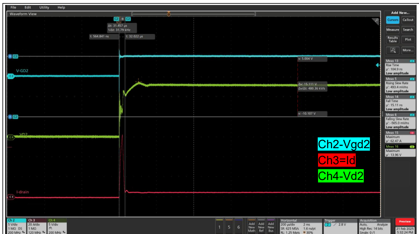
Figure 14 Turn on without RC delay on gate drive path- V_{D1}=20\text{ V} , I_d=5\text{ A} (load), V_{GD2} = 0\text{ V} to 5\text{ V} , I_{d\_max} = 62.47\text{ A} , t_{I\_max} = 32.6\text{ }\mu\text{s}
