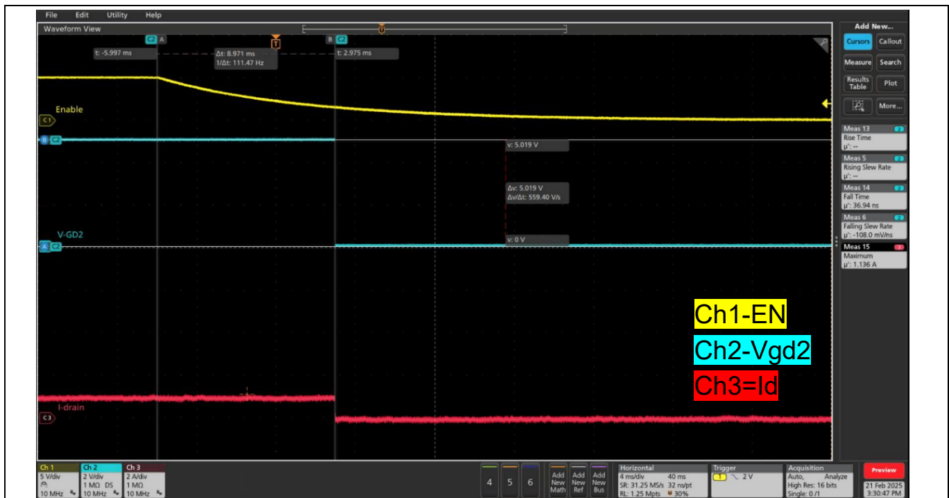
Figure 16 Turn off - V_{D1} = 5\text{ V} , I_d = 1\text{ A} (load), EN = 5\text{ V} to 0\text{ V} , V_{gd2} = 5\text{ V} to 0\text{ V} , t_{off} = 8.97\text{ ms}
