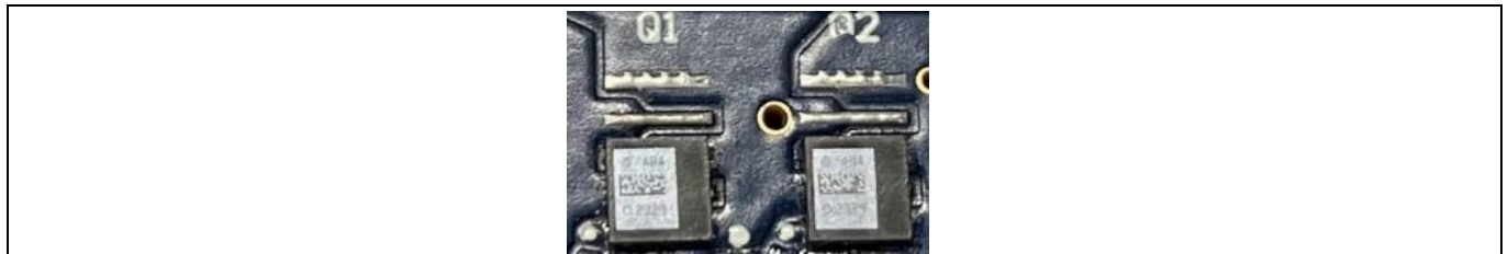
Figure 21 Reworked board with IGB110S10S1 assembled instead of IGC033S10S1
