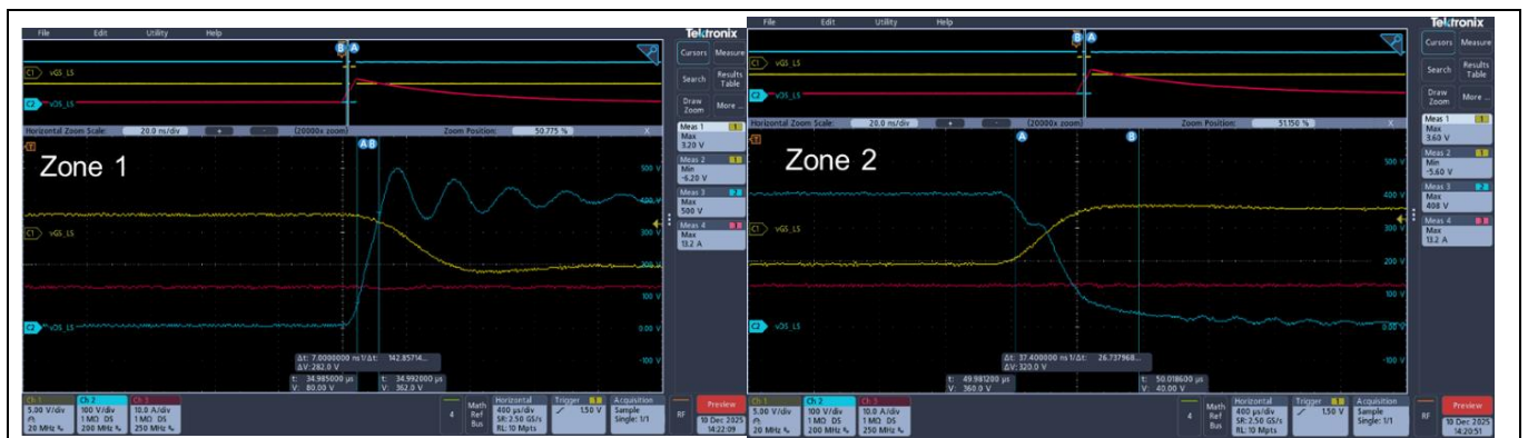
Figure 18 Double pulse test waveform in zone 1 and zone 2
