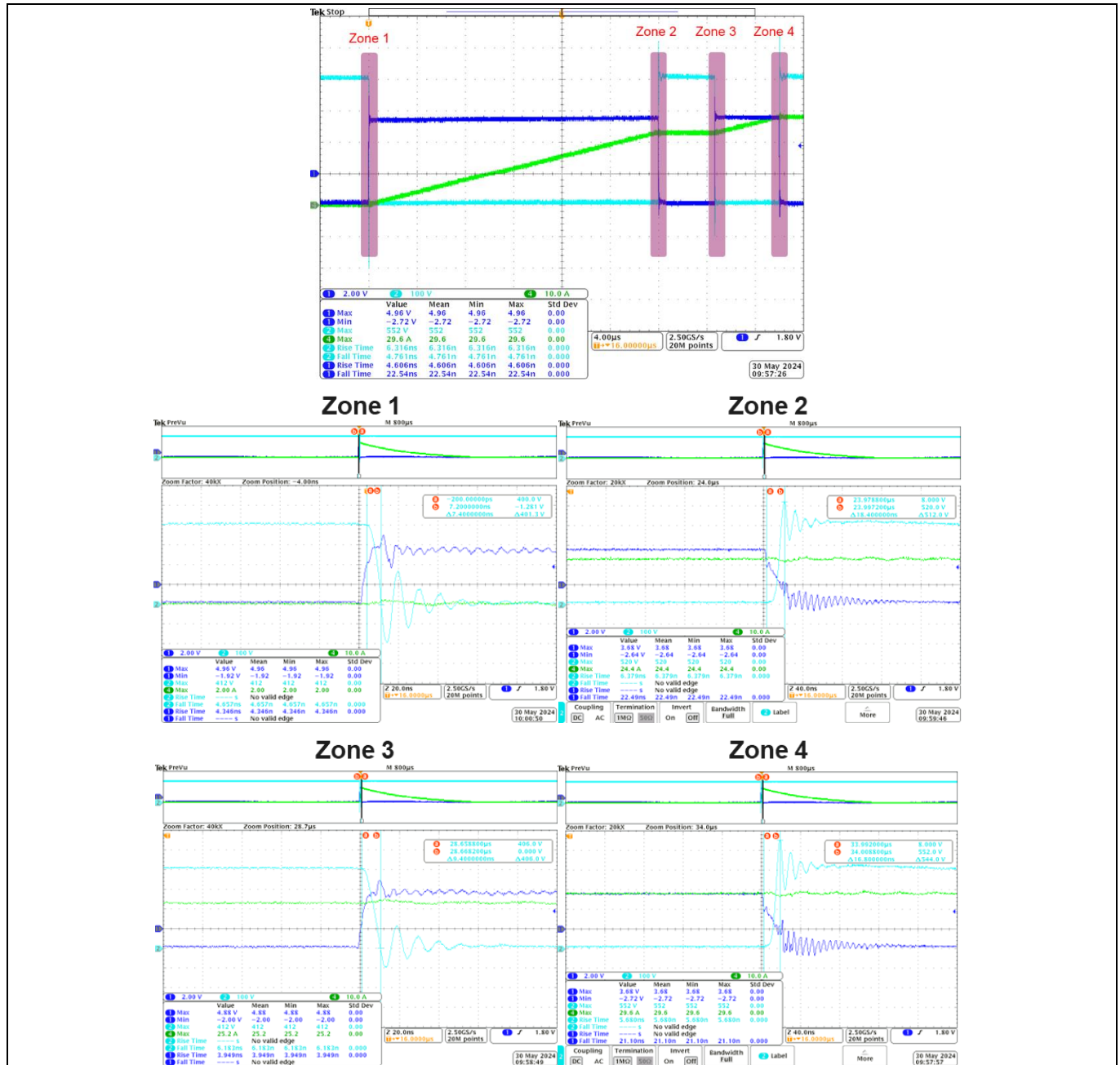
Figure 15 Double-pulse test waveform with single-channel isolated driver IC and isolated standby aux power circuit (IGT65R055D2)
