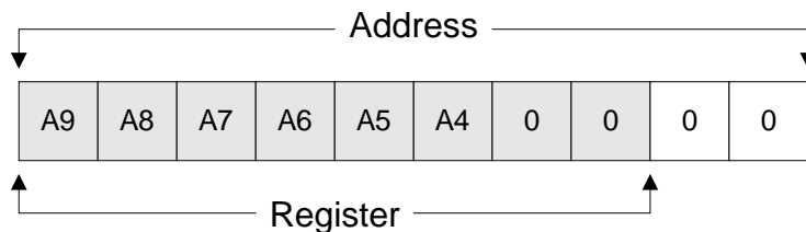
Figure 8-4. FIFO Start Address Format
