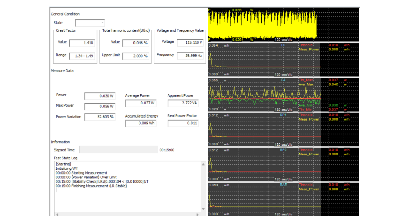
Figure 9 Detailed power measurement results @115Vac, 60 Hz
